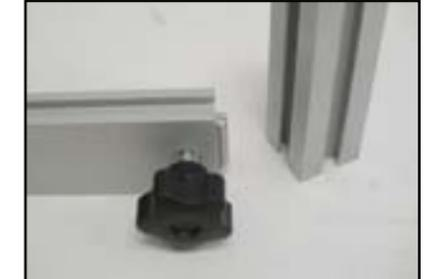
**Detail F:** Plastic Star Knobs are used to tighten locks where horizontal extrusions connect with vertical extrusions. Turn the knobs clockwise to tighten. Turn counter-clockwise to loosen, but do not remove knob.
