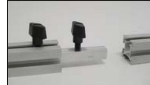
**Detail E:** A square connection bar with plastic T Knobs is inserted between two vertical extrusions joined end-to-end. Turn the knobs clockwise to tighten.
