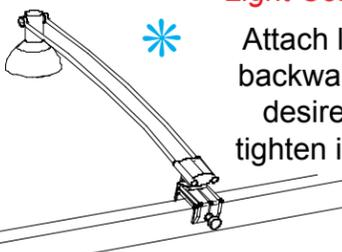
Attach lights to backwall where desired and tighten in place.
