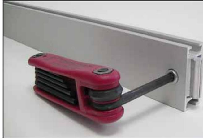
Detail A: Most horizontal extrusion connections have a patented expandable lock. This lock inserts into the groove of an opposing extrusion. Tightening the lock with the Hex Key Tool expands the lock and creates a strong positive connection.
