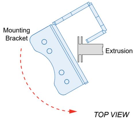
② Slide bracket forward, then down onto V4 connector.
